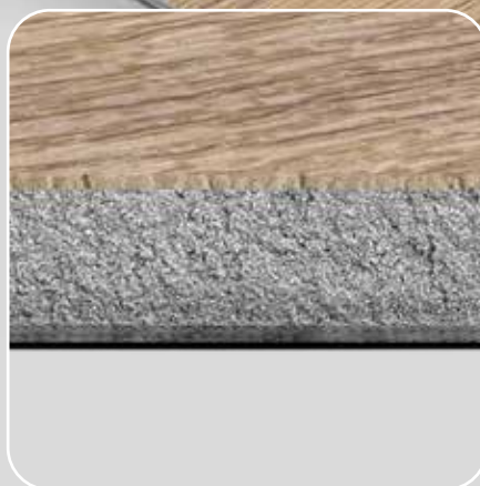
Denscore PRO mineral core manufactured by extruding calcium carbonate and additives; thickness: up to 4,5 mm
